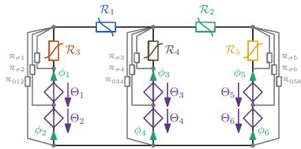
Fig. 3: Magnetic domain of the LE transformer model
