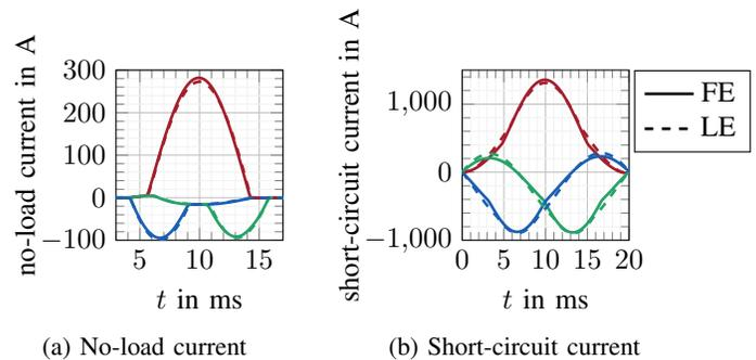
Fig. 7: Comparison of the primary current between FE and LE model
